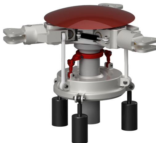
Fig 28: Ibis Main Rotor Hub and Swashplate
